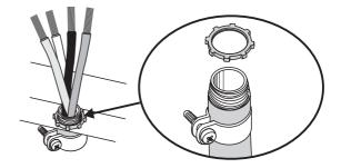
Fit a squeeze connector (not supplied with the range), to your conduit. Insert the conduit through the reducer plates on the mounting bracket. Allow enough slack to easily attach the wires to the terminal block.
